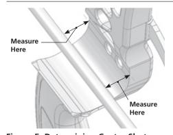
Center shot can be set by measuring from the back of the riser to the arrow and then from the front of the riser to the arrow. Once this is equal, you are at the approximate center shot of
