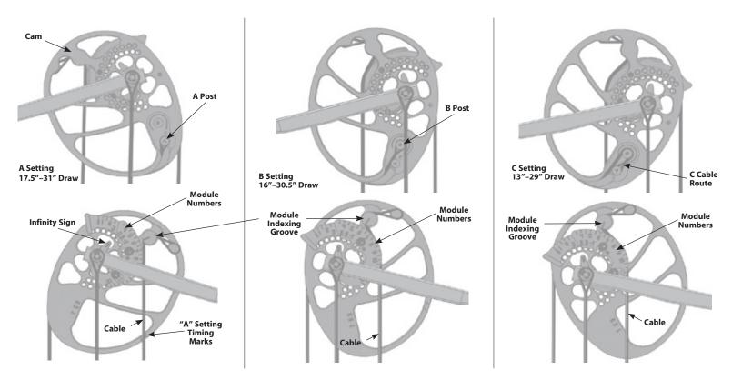
Figure 1. Diamond Infinite Edge Pro draw length adjustment.
